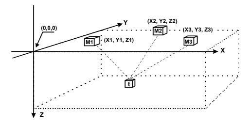
Network formation is entirely up to the user, just type the X,Y coordinates of each HX11TR device (labeled M). into a file called layout.hxm. The following is simple efficient setup with distances between monitors, everywhere the same.
