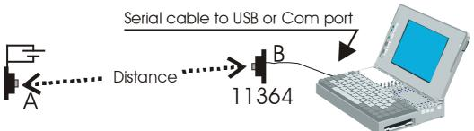
The images show an ultrasonic transponder wireless and a free moving point A. Through ultrasonic identity exchange, caller B measures the distance to transponder A, both directly and using a reflection of an orderly object.
