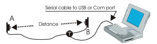
The images suggest a setup allowing ultrasonic identity signal to be transmitted from device A to device B or vice versa, or echoed of an orderly object. The receiving device reports the time elapsed from start (synchronization) until it receives the signal. Hence time of flight can be extracted from the receiver.
