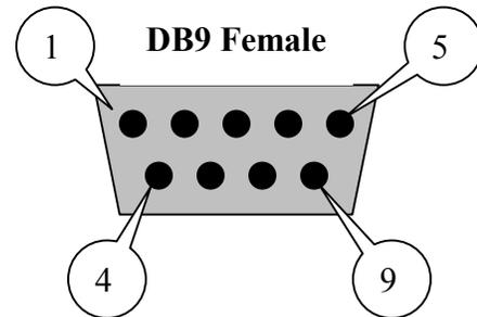
Pins on D-Subs 9 or 25 pins are always marked with the appropriate numbers for the pins as shown above.
